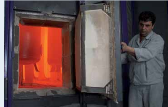
Tanks being porcelain-fired at Stiebel Eltron's factory in Holzminden, Germany
